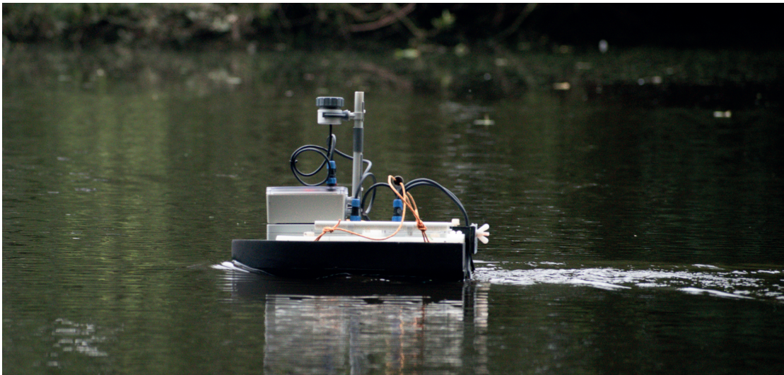
Fig. 1 This is a side view of the small sonar EVA boat measuring only 540 mm × 380 mm × 220 mm. The pod on the mast houses the UWB receiver.
